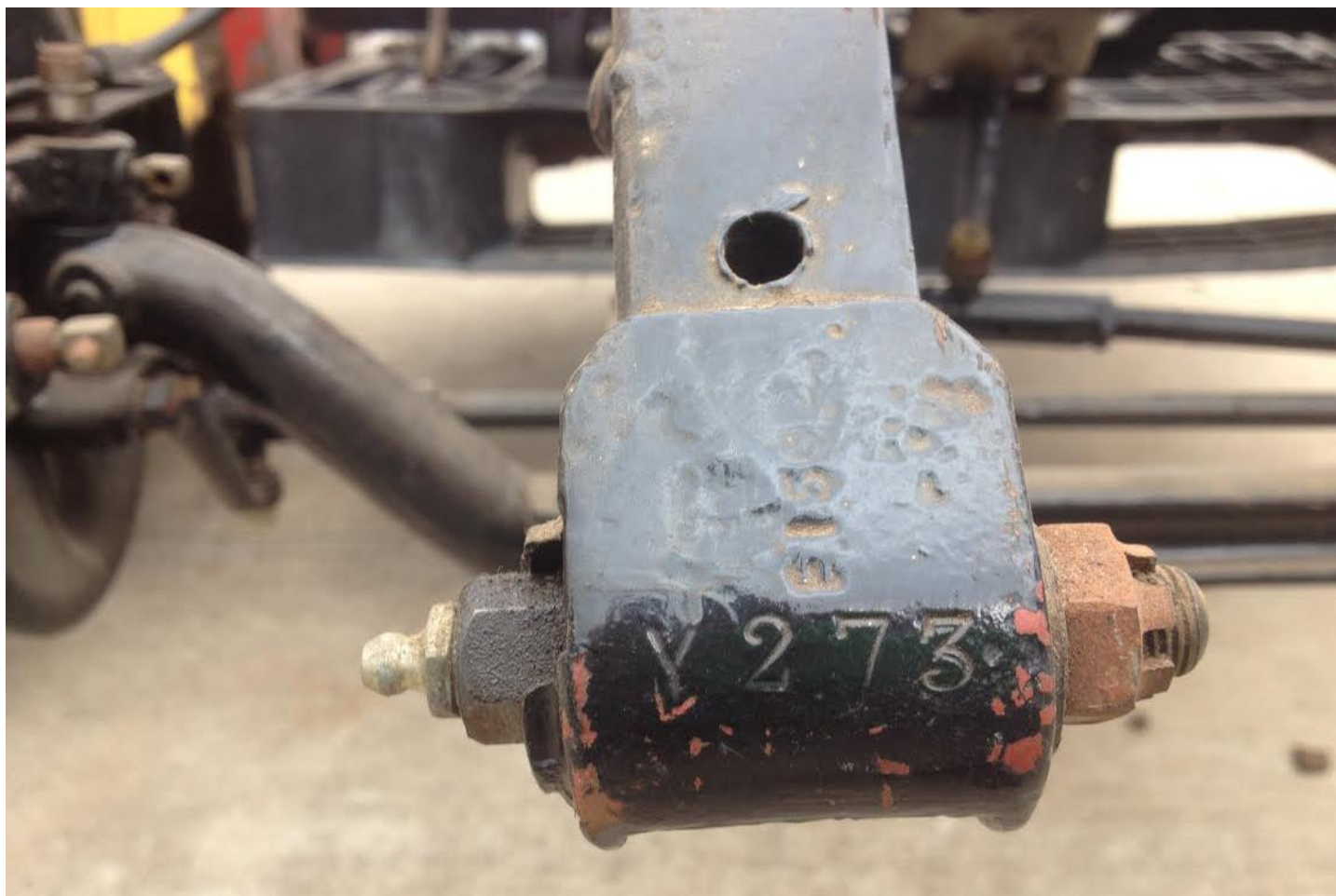
The chassis number Y273 clearly visible on the front dumbiron of Keith Fowlie's 1929 Minor chassis.
