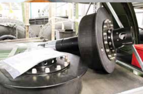
Lancaster brake hubs on a rack in the BBMF hangar, fitted with the pneumatic rubber brake bags but not with brake shoes. The hub on the right is attached to the wheel axle. The other brake hub would fit on the other end of the axle.
