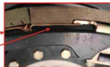
☒ Lancaster brake unit. There are 20 brake shoes per wheel, which are forced against the wheel hubs by a rubber brake bag inflated by pneumatic pressure.
