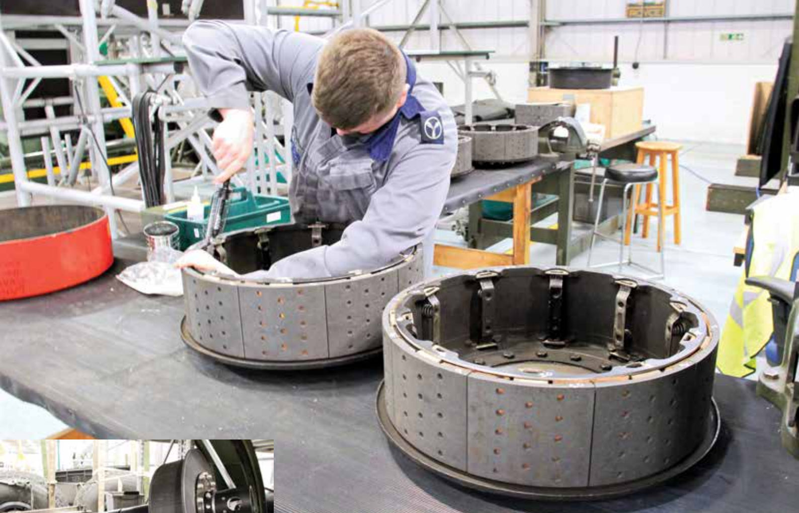
RAF BBMF technician SAC(T) Jack 'Buzz' Busby completing the fitment of the new brake shoes to the Lancaster brake hubs in the BBMF hangar in January 2020. (All photos this page: Clive Rowley)
