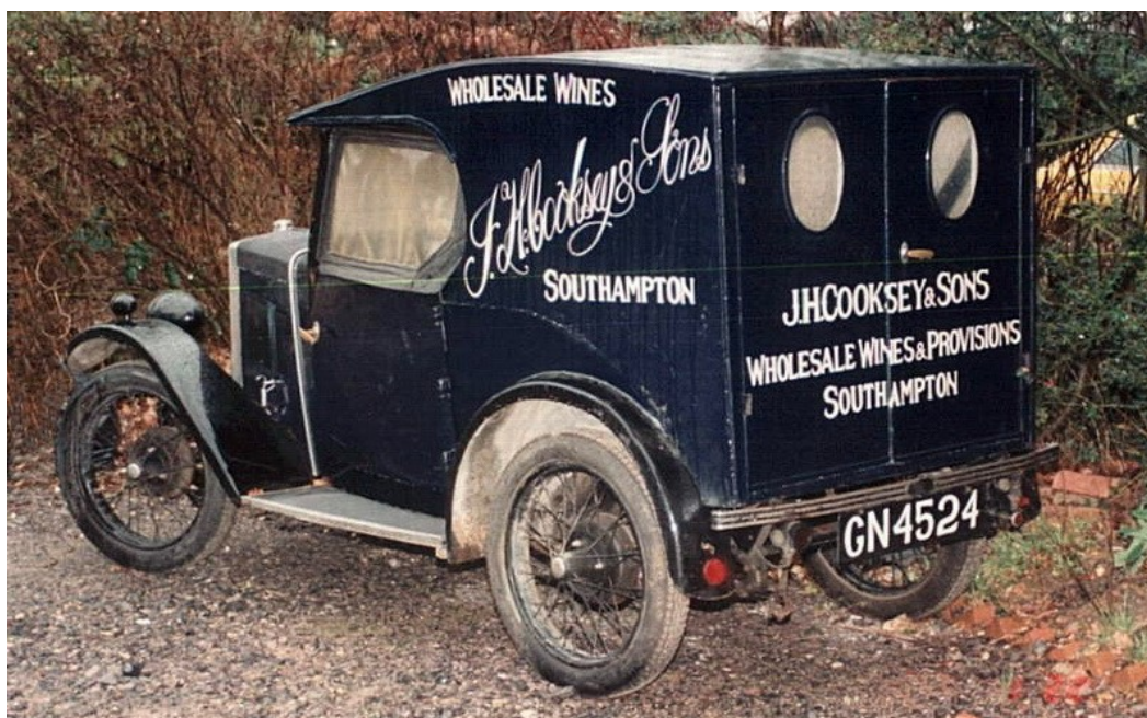
Minor Duple van/tourer GN 4524 (M27283) in van mode. The curve of the original tourer body can just be seen under the word Southampton.
